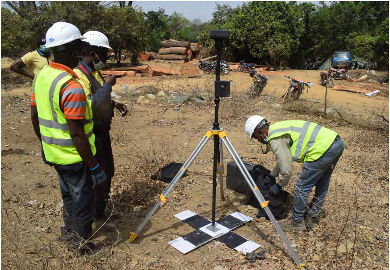
Figure 2.2: GhBC Field Survey Team setting up Drone Base Station at Ntereso on the Ghana-Côte d'Ivoire Boundary.
