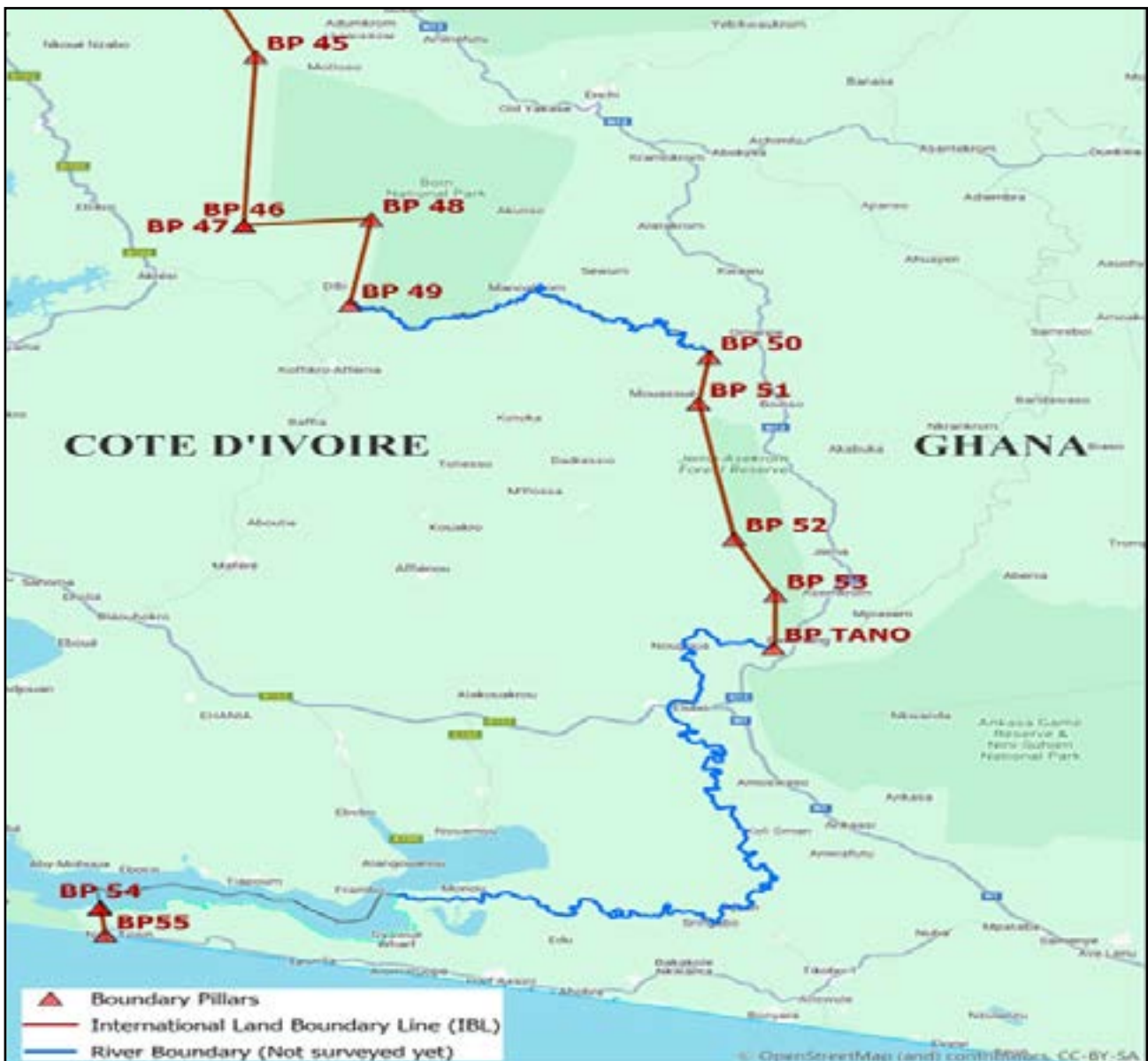
Figure 2.8: Map of Boundary Pillars Marked in Phase I of the Ghana/Cote d'Ivoire Land Boundary Reaffirmation (BP45 - BP55).
